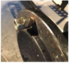
G. You will need to remove the 2 Stud on the axle, double nut tight the Stud as in photo & turn counter clockwise the inside nut. The stud should unscrew itself from the axle.
